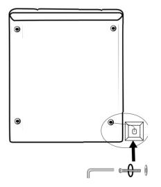
clockwise turning of Allen key for tighten of bolt
