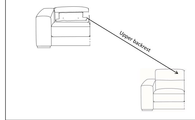
Step5: Tighten the upper backrest to the lower backrest of LHF Chair with bolts (f) and washers (g) by Allen key (e).
