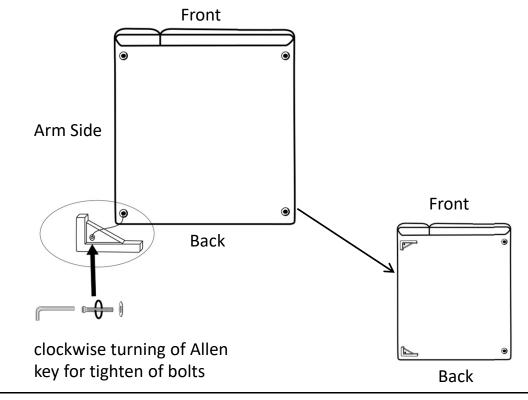
Step3: Tighten the plastic legs (b) to the bottom of LHF Chair with bolts (c) and washers (d) by Allen key (e).
