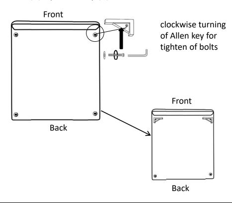
Step13: Tighten the plastic legs (b) to the bottom of RHF Terminal Chair with bolts (c) and washers (d) by Allen key (e).
